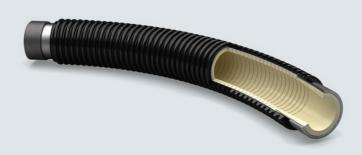
CERA SYSTEM supplies wear resistant flexible solutions. Ceramic hoses manufactured by CERA SYSTEM can be used everywhere where hoses regularly wear and must be replaced. The hose consists of ceramic rings that are vulcanised together with special reinforced rubber materials. Pressures of up to 10 bar / 145 psi are permitted.
